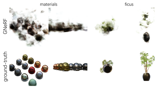
Fig. 13. 3D reconstruction results of GNeRF from unposed images. GNeRF fails in certain scenes, such as ficus and materials, because GNeRF may not initialize coarse poses when the images of a scene are highly similar.
